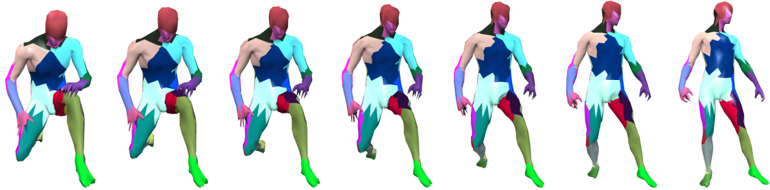
Figure 8. The images show a matching between the leftmost and rightmost models taken from the SHREC 2011 benchmark [1] by linearly interpolating between the triangle correspondences. This transition illustrates the geometric consistency property of the proposed method: At any time during the interpolation the model is a closed triangle mesh.
